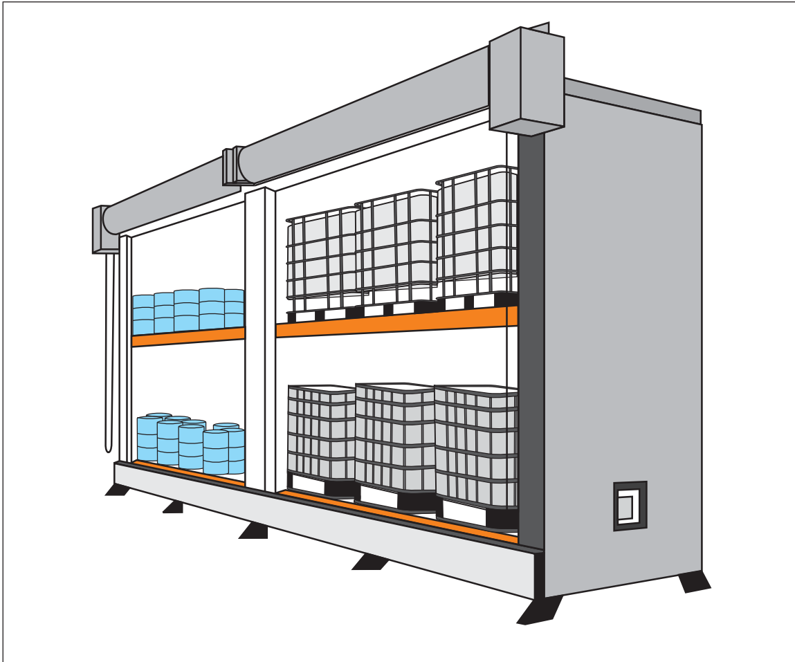
Fig. 2.2.3.2. Ignitable liquid storage locker
